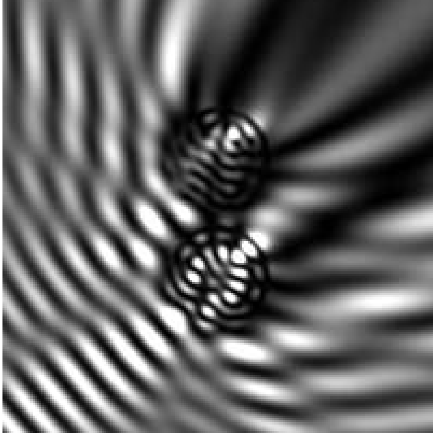
Figure B.6: This is an intensity plot of a light wave scattering off two thick lenses which has a higher index of refraction: n = 2.24 . Now, the focus in the lower lens is actually inside the lens. An plane wave is incident from the lower left corner. The intensity in the upper lens is irregularly shaped because it is partly in the shadow of the lower lens. This picture was generated using the methods presented in Chapter 4.
