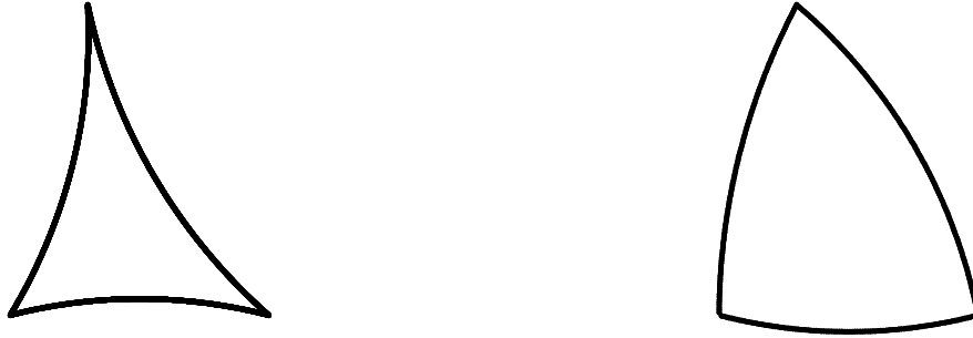
Figure 4.1: left Concave triangle and right convex triangle. The concave triangle is composed of 3 arcs of circles of radii 2.1, 2.2 and 2.3. The convex triangle is made of arcs of circles of radii equal to 2.0, 2.1 and 2.6.
